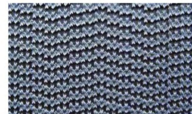
名称：波浪形高摩擦 代码：9 深度：2.4mm 宽度：3000mm 特性：表面摩擦大，适用斜面输送 行业：物流、机场等 Name:Wavy Super grip Code:9 Thickness:2.4mm Width:3000mm Property:Incline conveying, very high friction Application:Logistic, Airport
